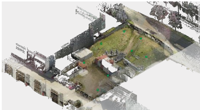
Fig. 5 Location of sensors on site
