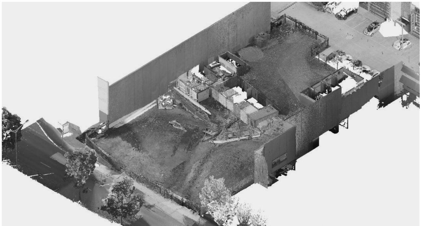
Fig. 7 Point Cloud of site 3D scanned
