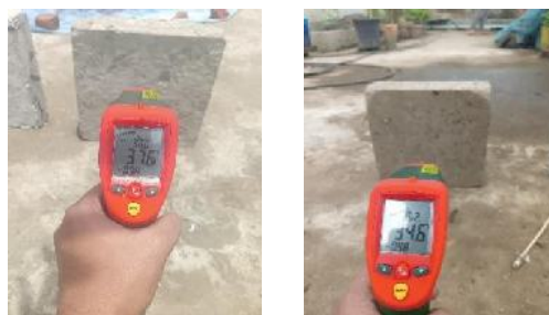
1 2 Time:4.00 P.M (1.Outer facade 2.Shaded facade)
