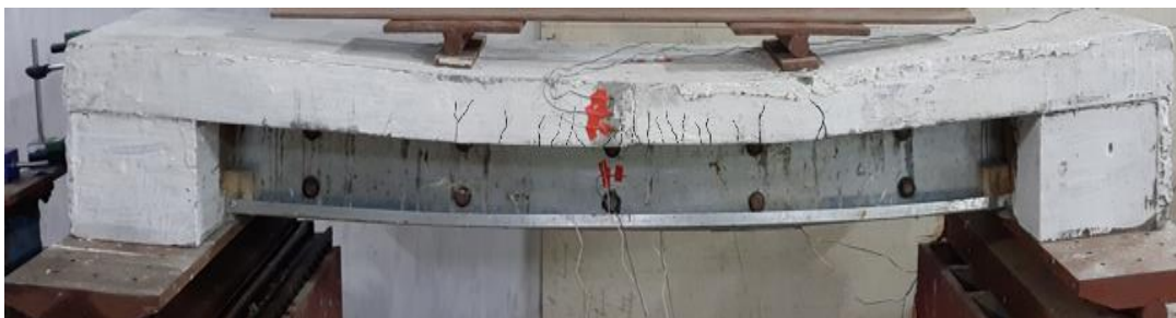
Figure 8 – Failure of Cold-formed steel-concrete composite beam under flexural loading
