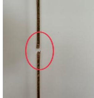
Figure 11: Failure at knot
