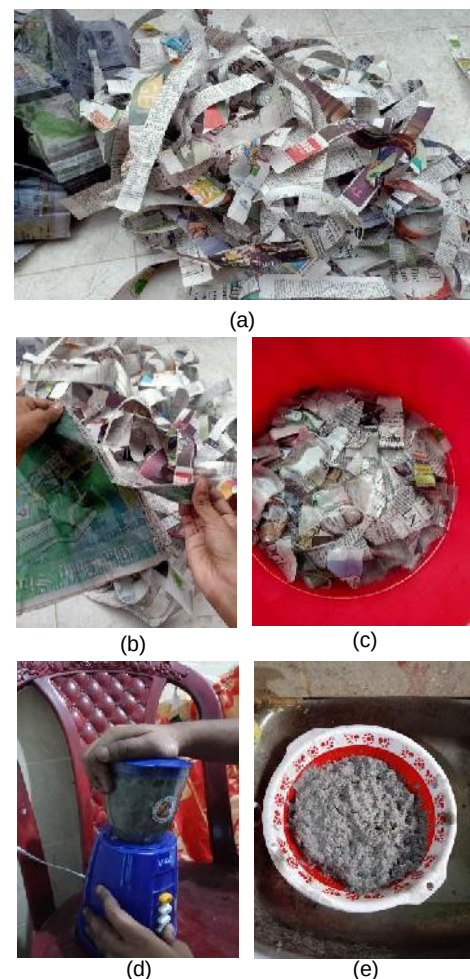
Figure 3: (a)Waste paper(b)Shredding, (c)Soaking, (d)Mixing, (e)Dewatering paper pulp
