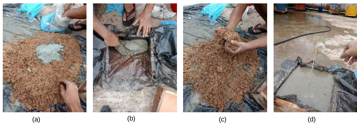
Figure 7: (a)Materials –gravel,sand,cement, (b)Mixing, (c)Filling up the mould, (d)Mould filled with concrete mixture
