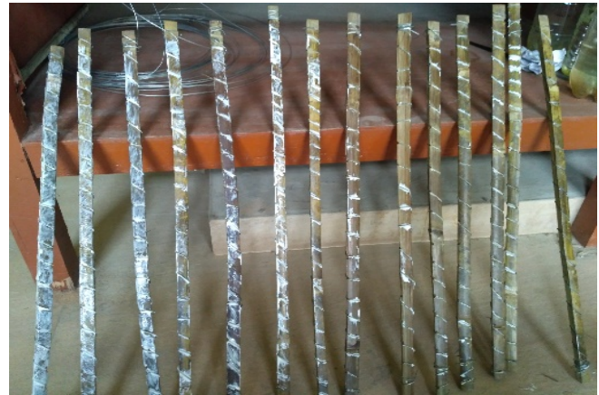
Fig 9 Epoxy coated GI wire rolled splints
