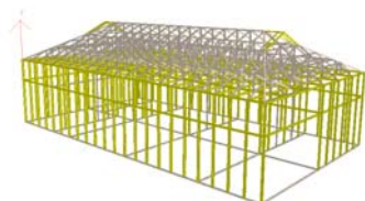
Figure 4.3 (a): CAD Model of LGS framing in Traditional Assam Type form
