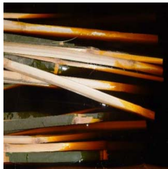
Fig 7 CCB treated splints
