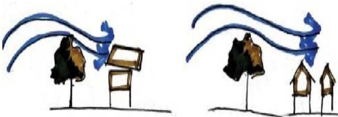
Figure 7: Orientation of roof in Majuli
