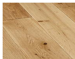
Figure 4.10 (b): Locally available compressed wood panels for flooring
