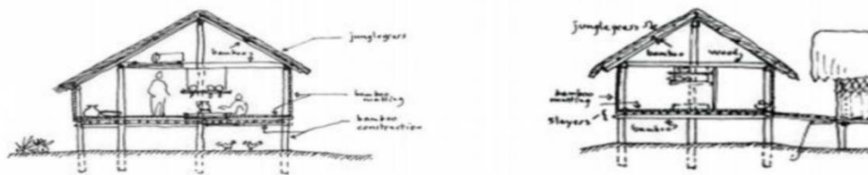
Figure 12: Side-sections of a Mishing house
