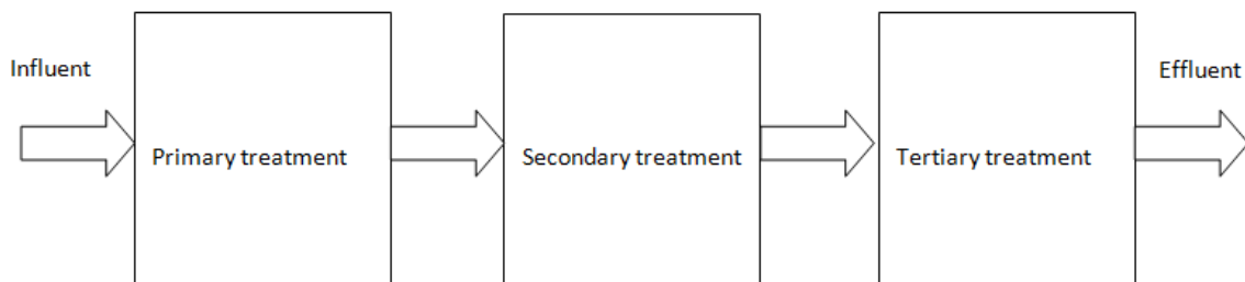
Figure 1. Block diagram representation of the three stages of wastewater treatment.
