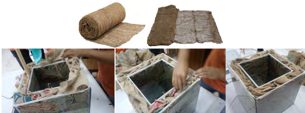
Figure 3: Local jute-fiber (sack) (top) and the cavity filled with jute-fiber/sacks (bottom)
