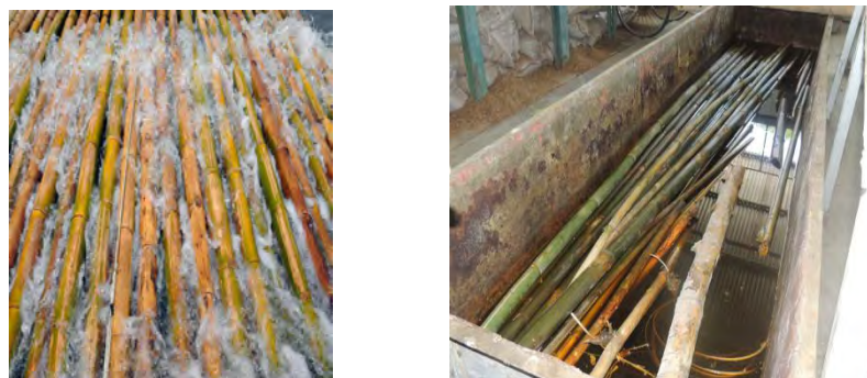
Figure 8: CCB treated bamboo in RFRI
