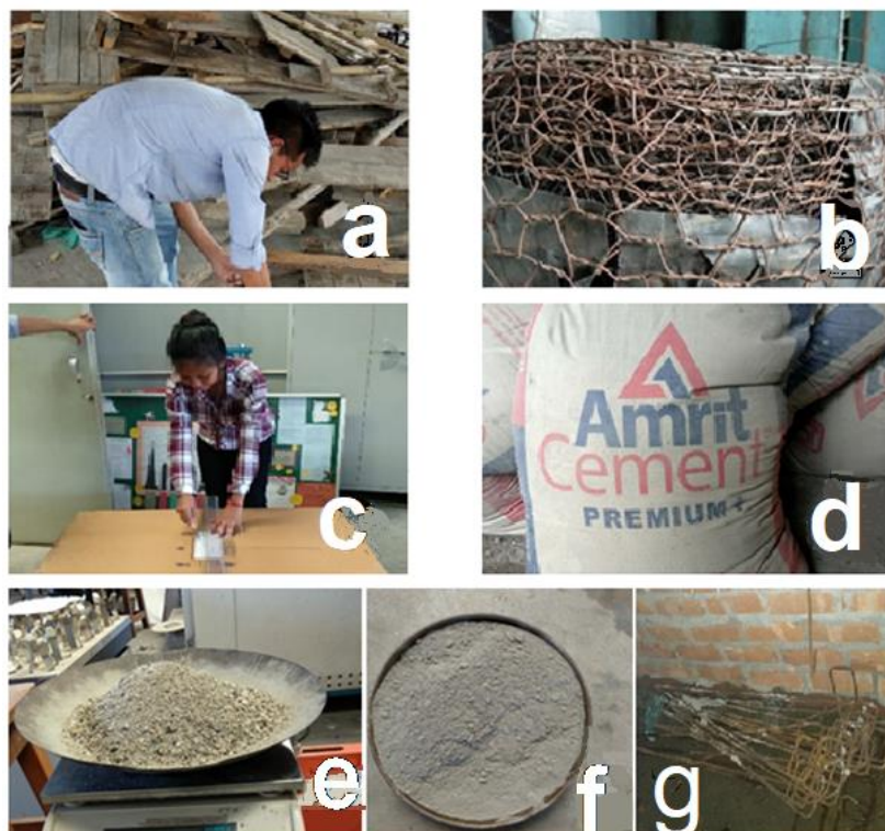
Figure 1: Materials for construction of ferrocement wall: a. Timber beign collected from construction wastes, b. Chicken Wire Mesh, c. Cardboard from construction wastes, d. Cement, e Sand, f. Fly Ash, g. Rebars from construction wastes
