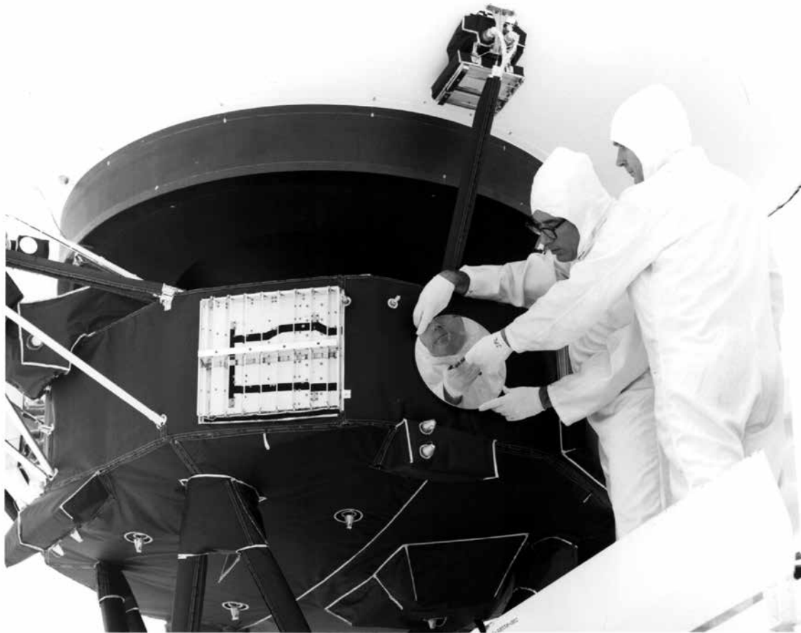
FIGURE 1 Voyager Interstellar Record being fixed to the Voyager 1 space probe prior to its launch in 1977. (Image Source: NASA: https://solarsystem.nasa.gov/galleries/voyager-1-gold-plated-record/ .)
